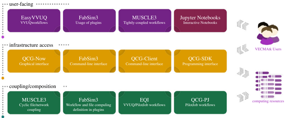
Figure 1. Overview of the main components, and their role within the VECMA toolkit. (Online version in colour.)
