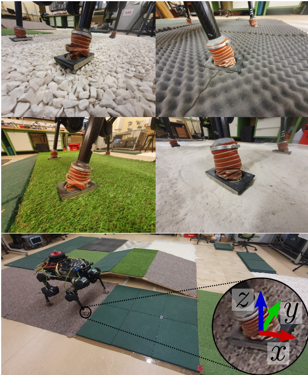
Figure 4.10: Top: Examples of foot positioning when collecting data on different terrains under controlled laboratory conditions. Bottom: Experiment 3: ANYmal with sensorized flat feet standing on the multiple terrain type course. Close up of the foot is provided. An IMU and fore/torque sensor is located in the sole with coordinate frame shown.
