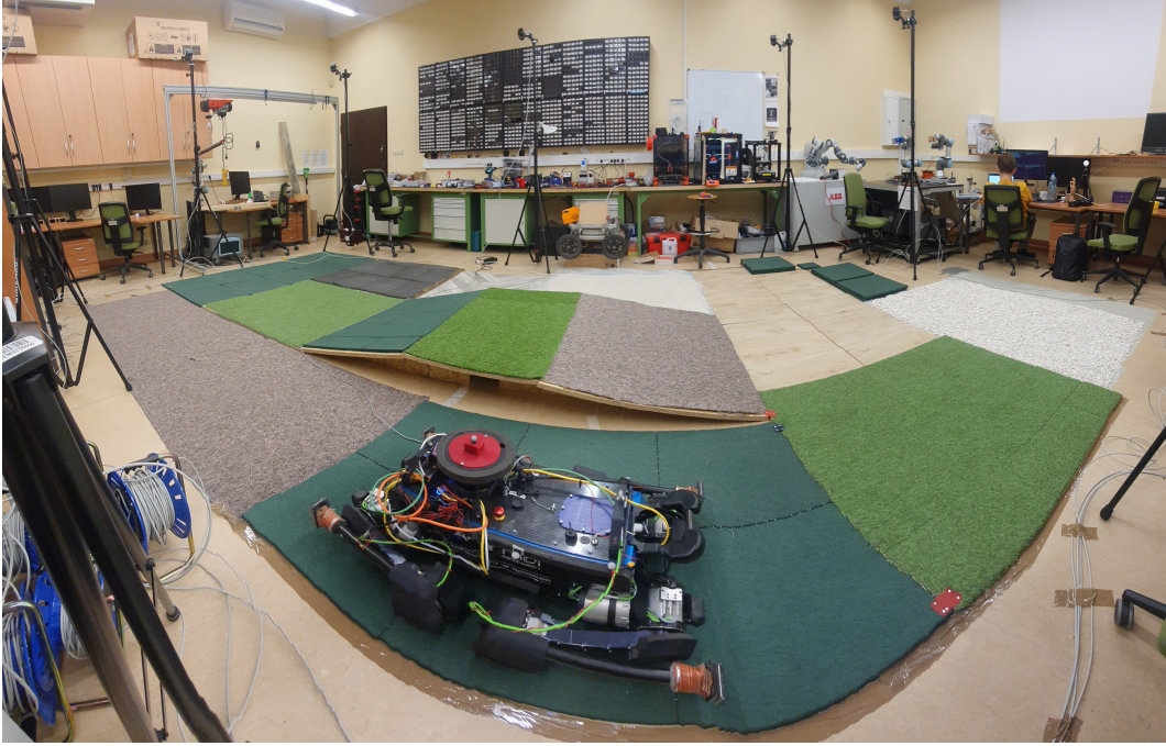
Figure 2.2: The experimental setup featuring the ANYmal robot in a custom-built environment equipped with an OptiTrack motion capture system built for the purpose of evaluating the localization system (Chapter 4). The large-scale scene contains diverse terrain types to facilitate repetitive haptic experiments.
