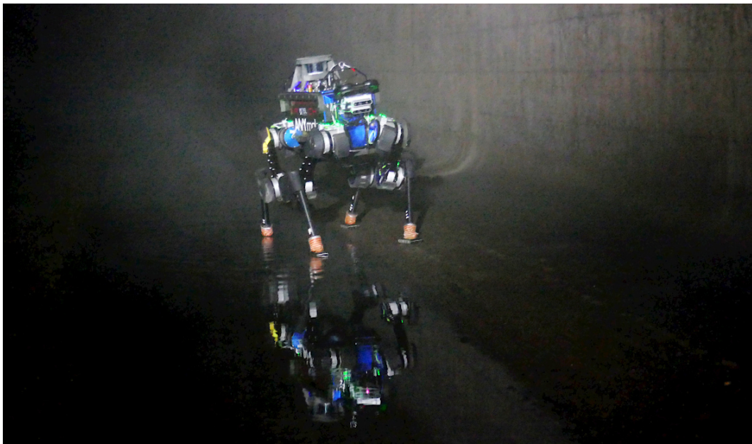
Figure 4.1: An ANYmal robot (Hutter et al., 2016) in a sewer with two feet in a slippery, wet depression and two feet in a dry, elevated area. With prior information about terrain type and geometry, it is possible for the robot to localized in the world using only touch. This would be extremely useful in dark and foggy environment (Image courtesy of RSL/ETH; Kolvenbach et al., 2020).
