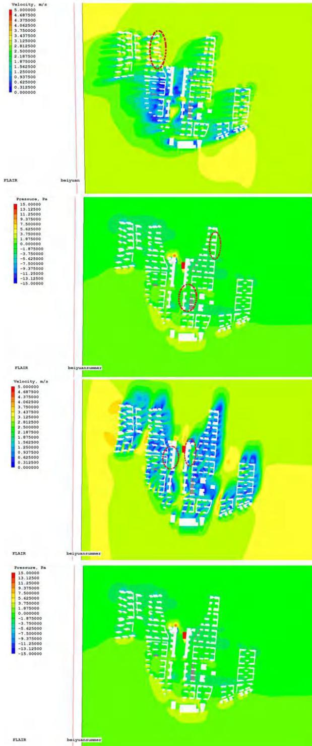
In winter, the prevailing wind direction and wind speed are the distribution map of wind speed at pedestrian height.
