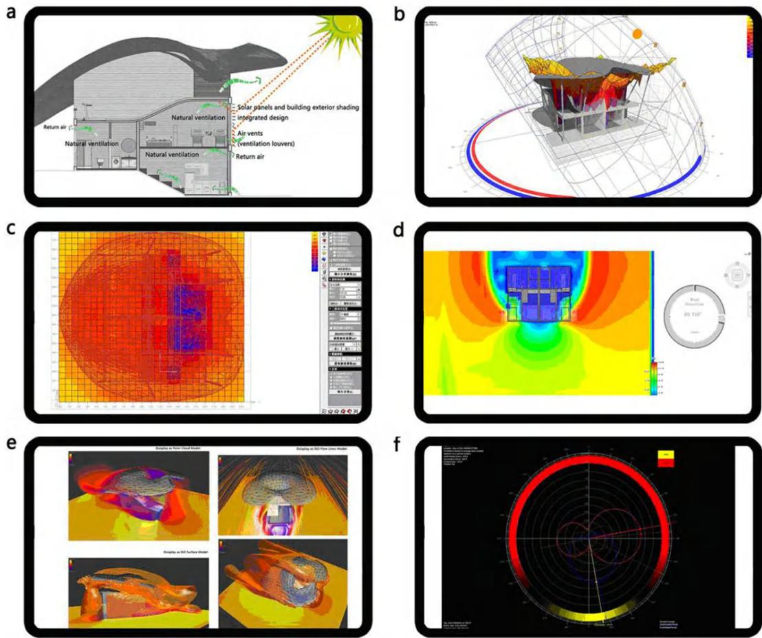
Figure 43. Schematic diagram of wind environment analysis (a) Natural ventilation analysis. (b) Natural lighting; (c) Natural lighting; (d) Wind environment simulation; (e) Wind analysis; (f) Best orientation. (Author design)
