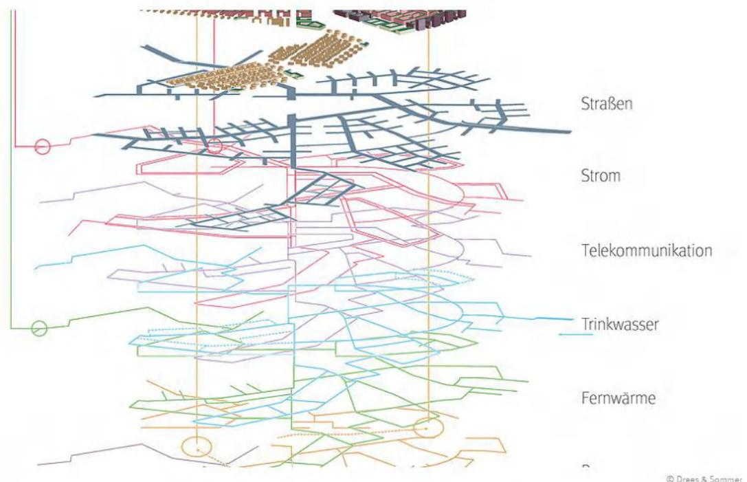
Figure 39. City BIM is the logical extension of Building Information Modeling to use in urban development. Source: <https://www.dreso.com/en/press/press-releases/2016/international-financial-center-in-moscow/>
