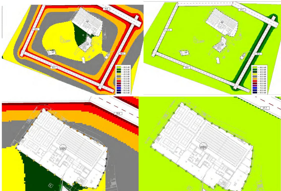
Figure 45. Distribution of sound pressure around the construction project. (Xiaolei Wang, Shandong Tongyuan Digital Technology Co., Ltd.)
