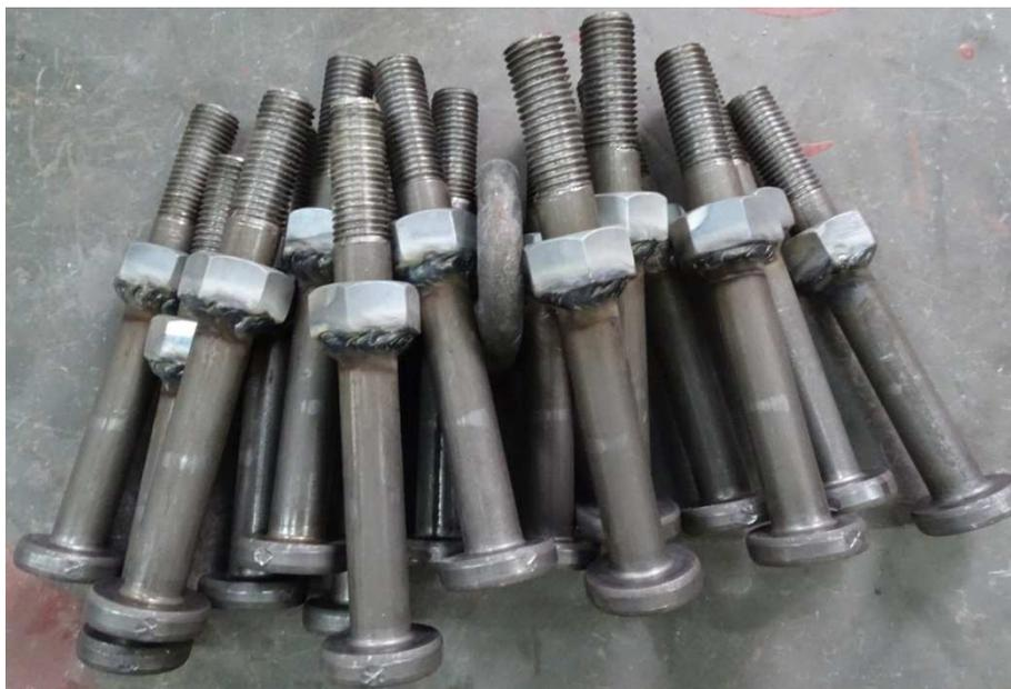
Figure 2.5. Prototypes of the shear connectors for aluminium-concrete composite beams
