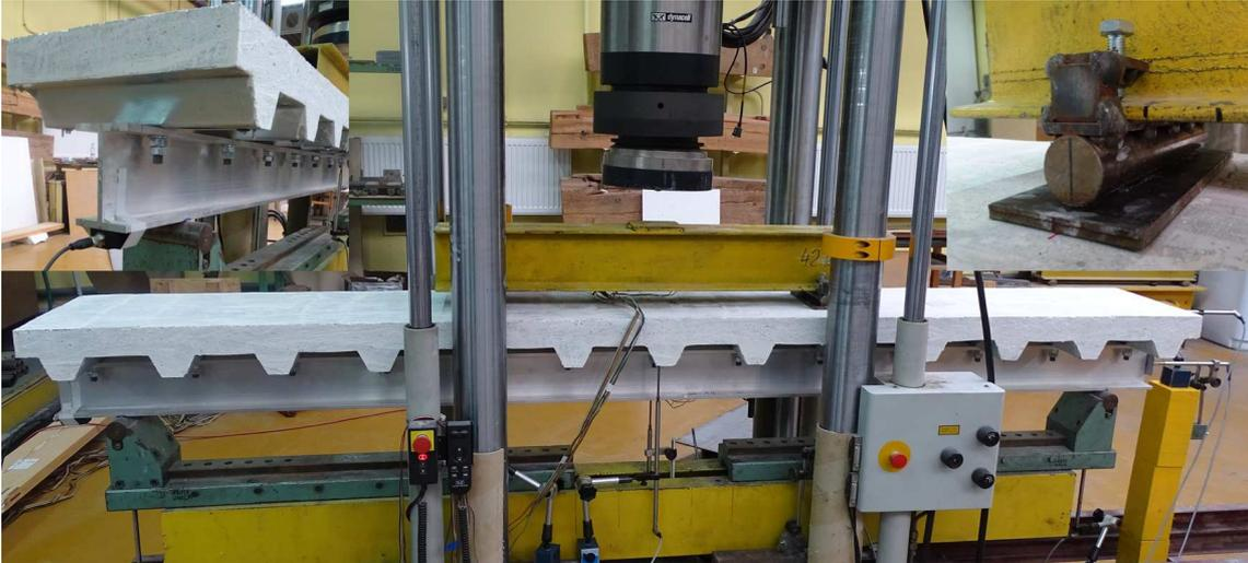
Figure 4.11. The specimen with the spreader beam
