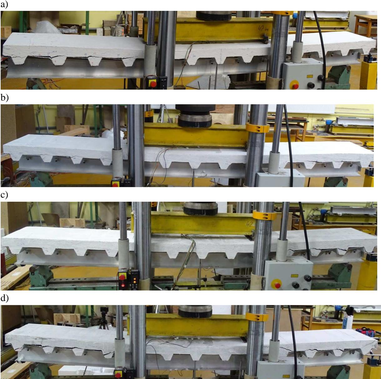
Figure 5.13. Beams at failure load: a) beam 1, b) beam 2, c) beam 3, d) beam 4
