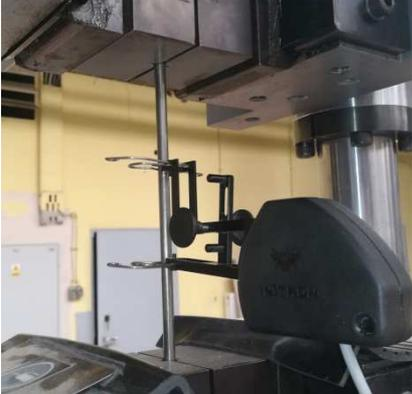
Figure 4.1. Metal specimens: a) the geometry of the flat samples; b) flat samples; c) round samples; d) tensile test on the flat sample; e) tensile test on the round sample
