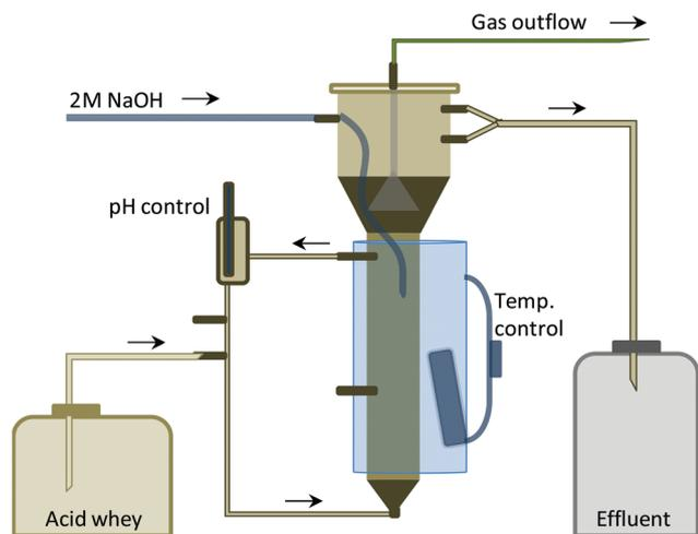
Fig. 1 Scheme of the upflow anaerobic sludge blanket reactor configuration.
