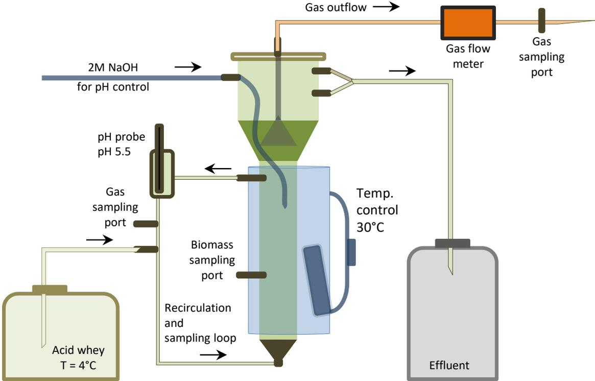
Fig. S1. Scheme of the reactor configuration, adapted from (Duber et al., 2018).
