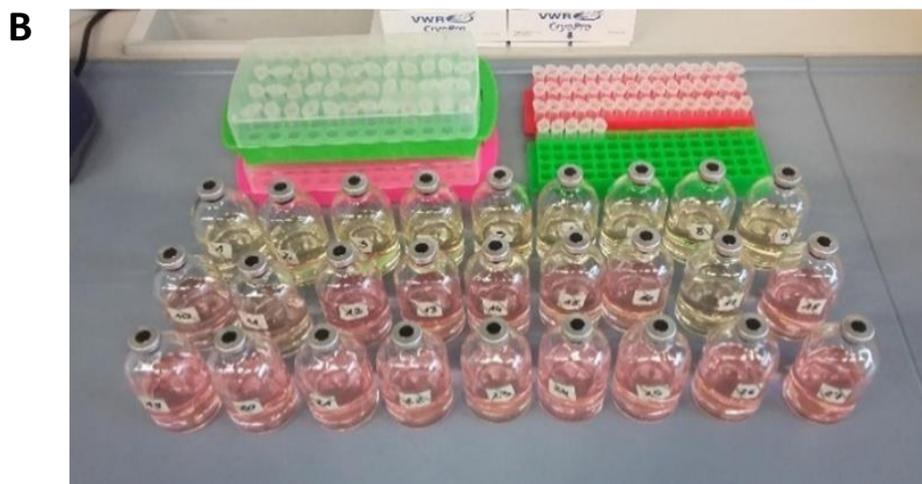
**Figure 4. A.** Scheme of serum bottle bioreactors for the batch mode fermentation processes and **B.** Bottles prepared for the batch mode experiment.
