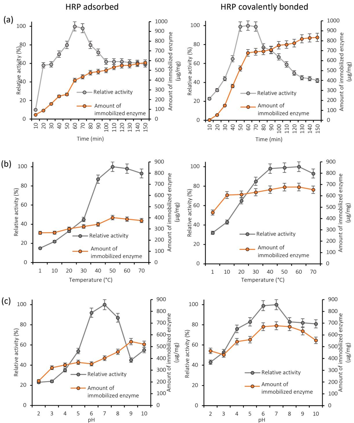
**Figure 20.** Effect of: (a) time of process, (b) temperature and (c) pH of immobilization on relative activity and amount of immobilized horseradish peroxidase onto nylon 6 fibers using adsorption and covalent binding methods.
