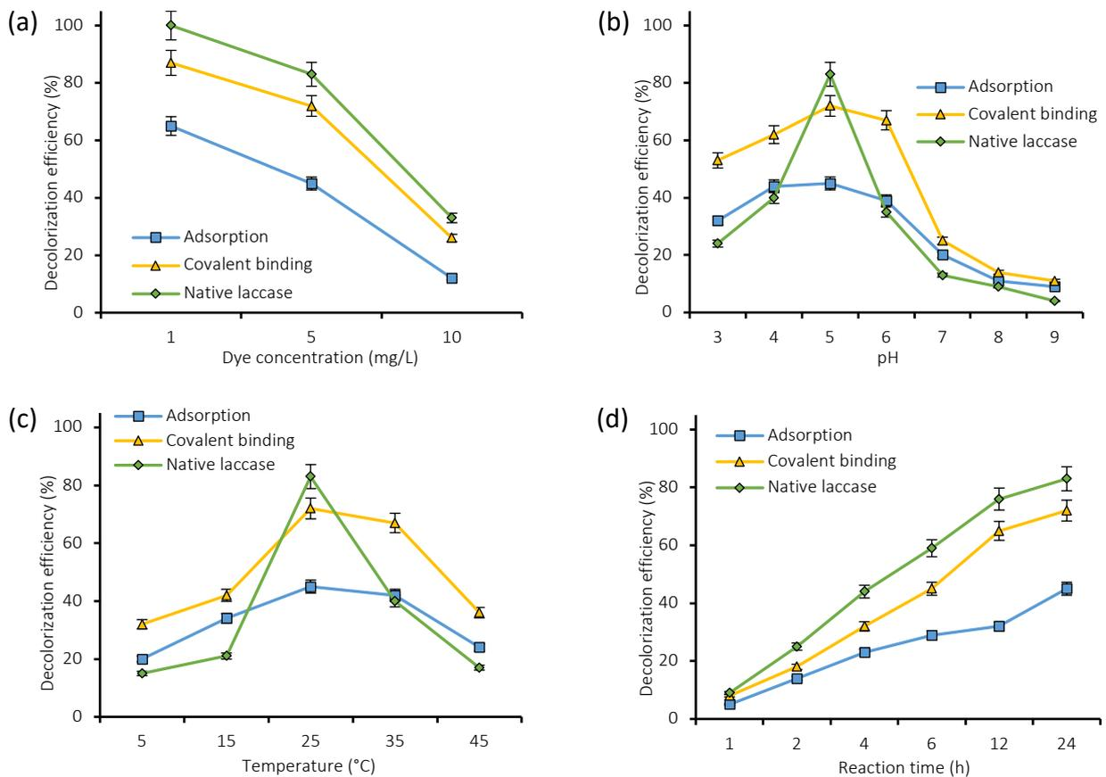
**Figure 17.** Effect of: (a) dye concentration, (b) pH, (c) temperature and (d) reaction time on decolorization efficiency of RB5 using laccase adsorbed and covalently bonded onto nylon 6 electrospun fibers.
