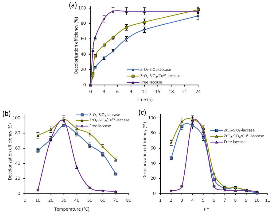
**Figure 14.** Effect of: (a) time of the process, (b) temperature and (c) pH on C.I. Reactive Blue 19 decolorization efficiency. The processes were carried out using ZrO<sub>2</sub>-SiO<sub>2</sub> and ZrO<sub>2</sub>-SiO<sub>2</sub>/Cu<sup>2+</sup> systems with immobilized laccase. The initial dye solution concentration was 50 mg/L.
