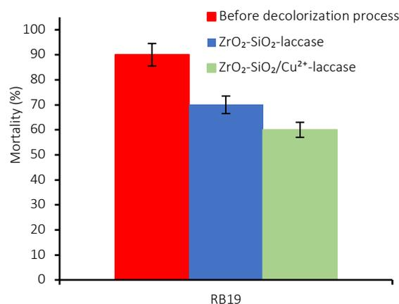
**Figure 15.** Mortality of *Artemia salina* larvae in the RB19 solution before and after treatment by  $ZrO_2-SiO_2$  and  $ZrO_2-SiO_2/Cu^{2+}$  systems with immobilized laccase.
