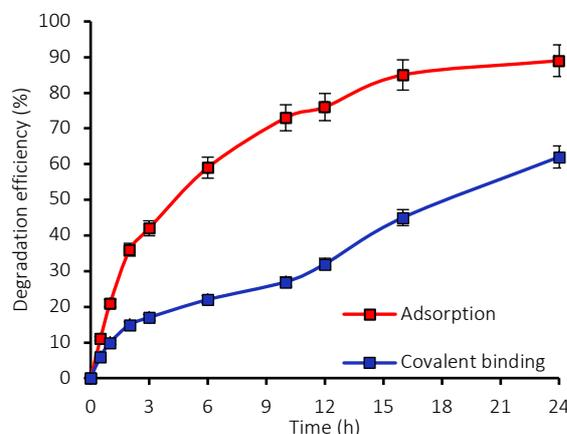
**Figure 25.** Decolorization efficiency of RB19 dye after process using systems made of PMMA/PANI fibers and adsorbed and covalently bonded laccase.
