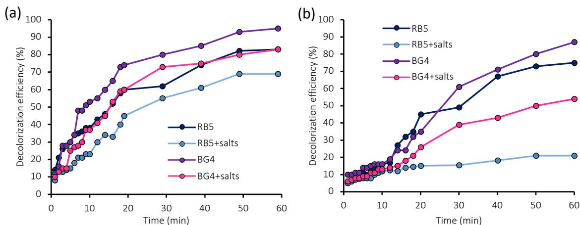
**Figure 22.** Decolorization efficiency of dyes from model aqueous solutions obtained after a process catalyzed by: (a) HRP adsorbed and (b) covalently bonded onto nylon 6. Reactions were carried out with the presence 1 mM of  $H_2O_2$ . Error values do not exceed 8%.
