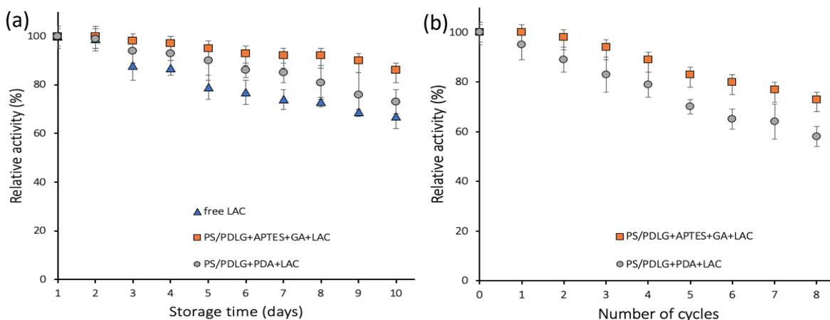
**Figure 28.** Effect of: (a) storage time and (b) number of consecutive reaction cycles on activity of laccase immobilized onto PS/PDLG+APTES+GA and PS/PDLG+PDA systems.
