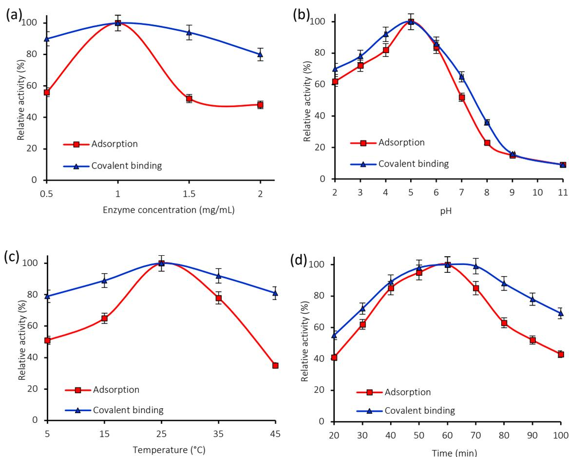
**Figure 23.** Effect of immobilization conditions on relative activity of laccase immobilized onto PMMA/PANI hybrid electrospun fibers by adsorption and covalent binding: (a) enzyme concentration, (b) pH, (c) temperature and (d) time of process.
