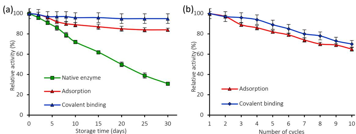
**Figure 24.** (a) Storage stability over 30 days of storage and (b) reusability over 10 consecutive catalytic cycles of laccase adsorbed and covalently bonded onto PMMA/PANI fibers.
