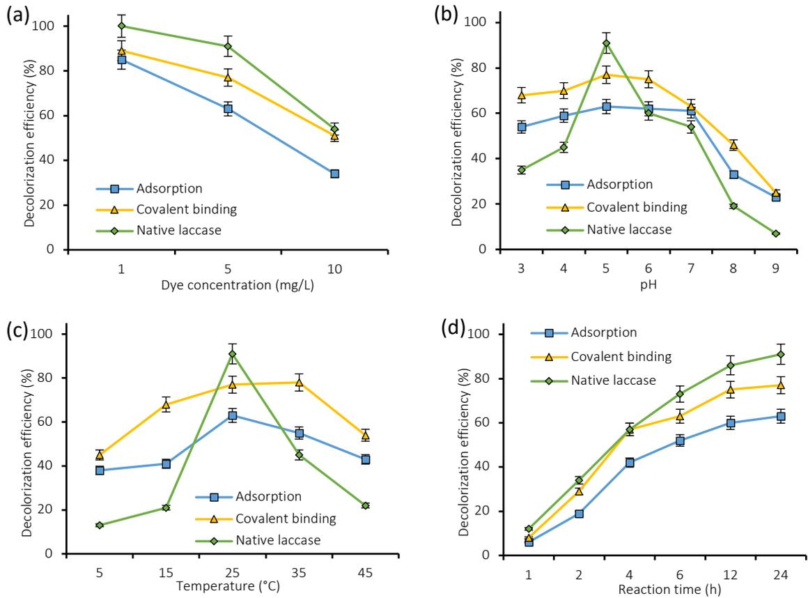
**Figure 18.** Effect of: (a) dye concentration, (b) pH, (c) temperature and (d) reaction time on decolorization efficiency of RB4 using laccase adsorbed and covalently bonded onto nylon 6 electrospun fibers.
