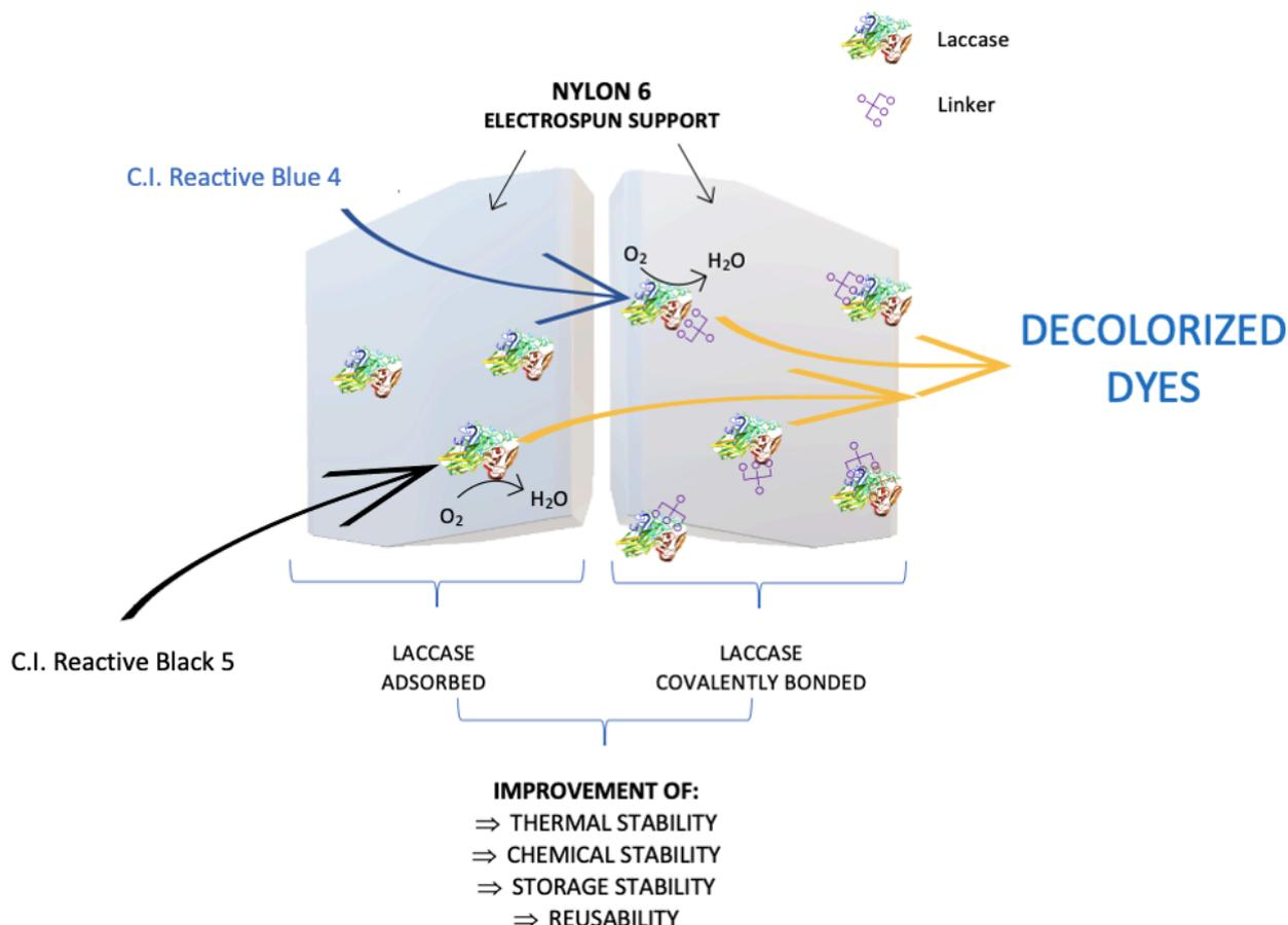
**Figure 16.** The schematic presentation of RB4 and RB5 removal by laccase immobilized by adsorption and covalent binding methods onto nylon 6 electrospun support.
