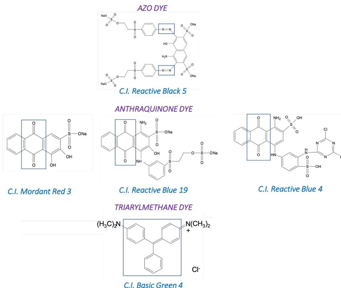
**Figure 11.** Dye groups most commonly applied in the industry with dyes examples and chromophores marked in their structures.
