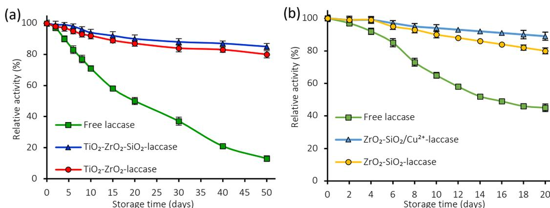
**Figure 13.** Storage stability of: (a)  $\text{TiO}_2\text{-ZrO}_2\text{-SiO}_2\text{-laccase}$  and  $\text{TiO}_2\text{-ZrO}_2\text{-laccase}$  and (b)  $\text{ZrO}_2\text{-SiO}_2/\text{Cu}^{2+}\text{-laccase}$  and  $\text{ZrO}_2\text{-SiO}_2\text{-laccase}$ , as well as storage stability of free enzyme.
