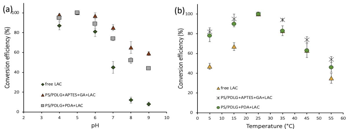
**Figure 27.** Effect of: (a) pH and (b) temperature on ABTS conversion efficiency catalyzed by free laccase and laccase attached onto PS/PDLG fibers via APTES+GA and PDA approaches, separately.
