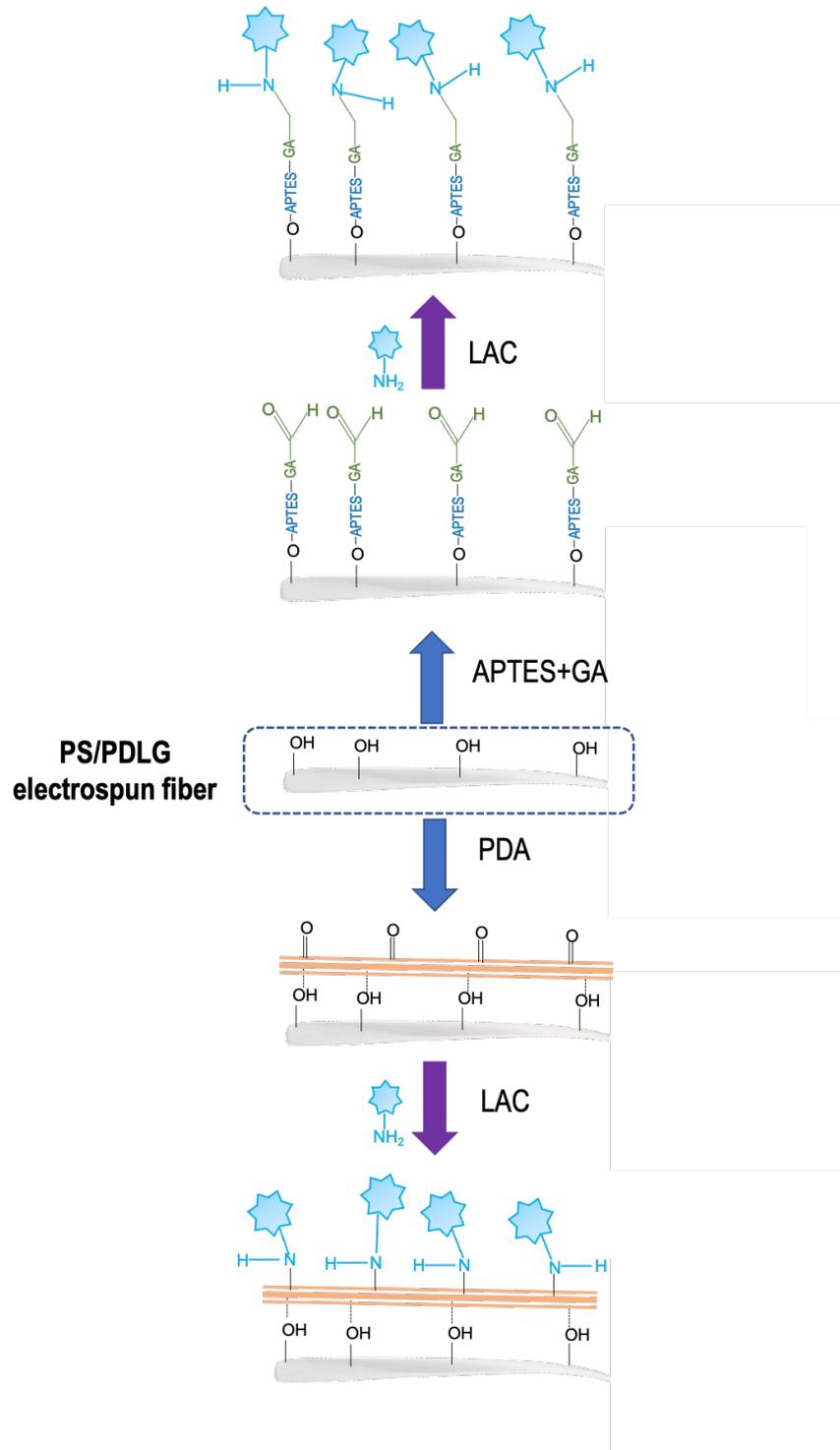
**Figure 26.** Mechanisms of laccase (LAC) immobilization via APTES+GA and PDA approaches onto PS/PDLG electrospun fibers.
