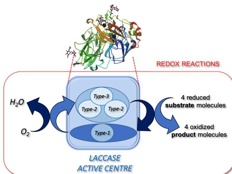
**Figure 3.** Scheme of redox reactions catalyzed by laccase indicating the presence of copper atoms (Type-1, Type-2 and Type-3).
