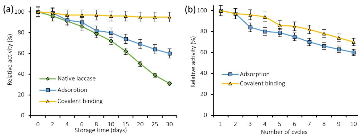
**Figure 19.** (a) Storage stability and (b) reusability of laccase adsorbed and covalently bonded onto nylon 6 fibers.
