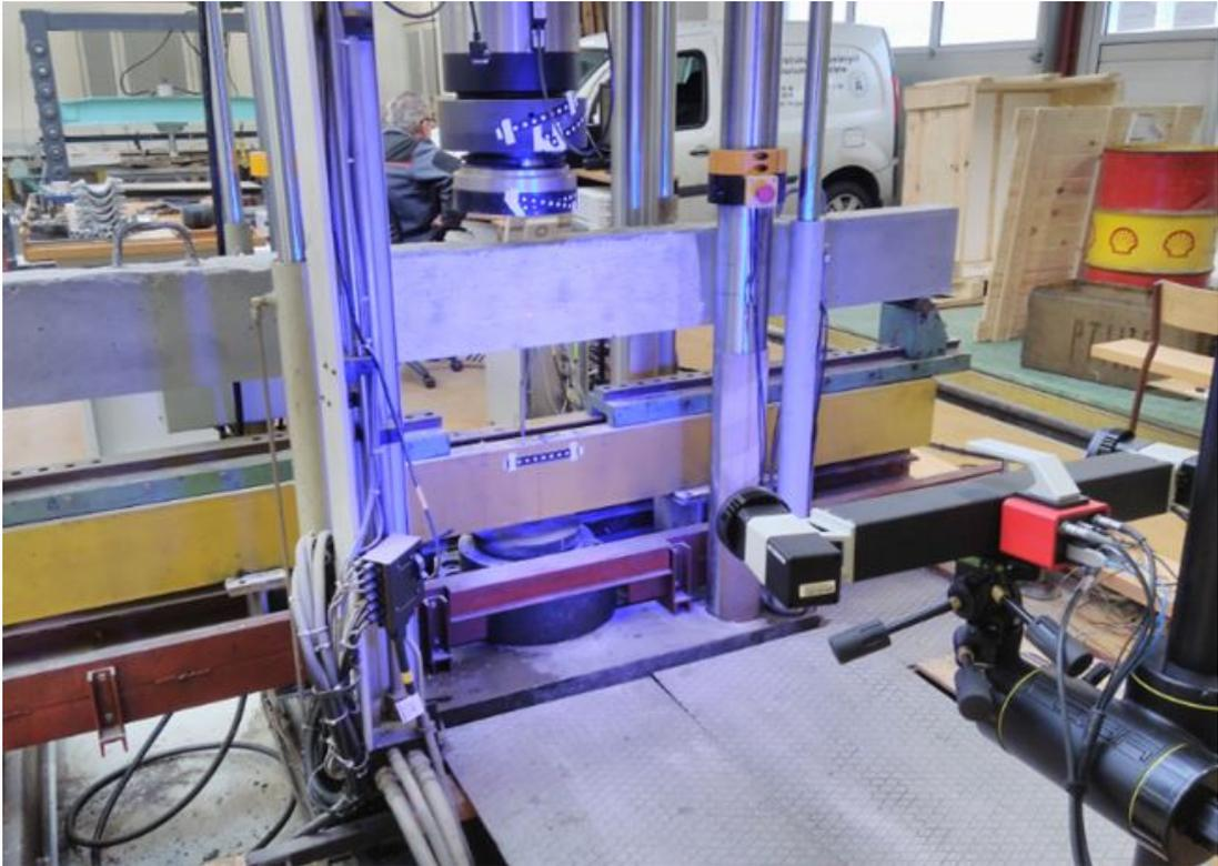
Fig. 4.55: The ARAMIS system during testing of full-scale beam
