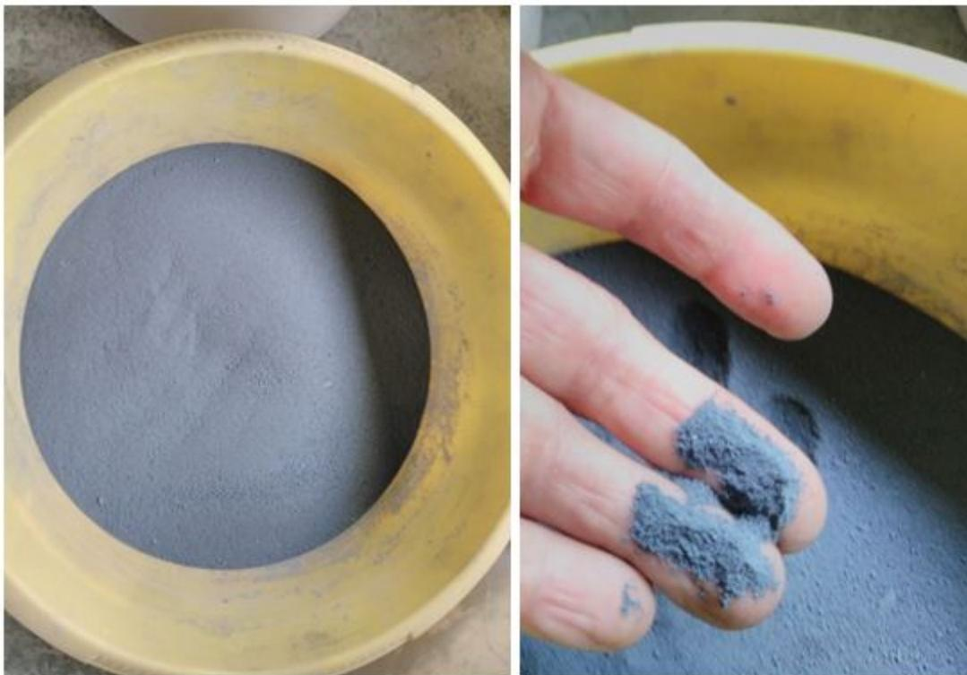
**Fig. 4.8:** Silica fume used in the research
