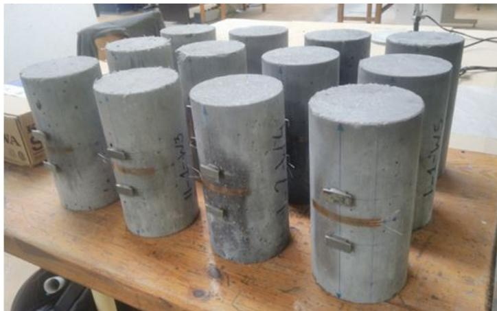
**Fig. 4.28:** Cylinder specimens for testing of material parameters
