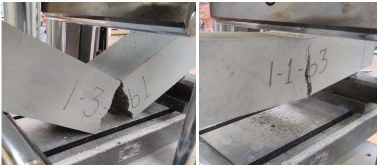
**Fig. 4.37:** The failure mechanism of beam without (on the left) and with (on the right) polypropylene fibre reinforcement
