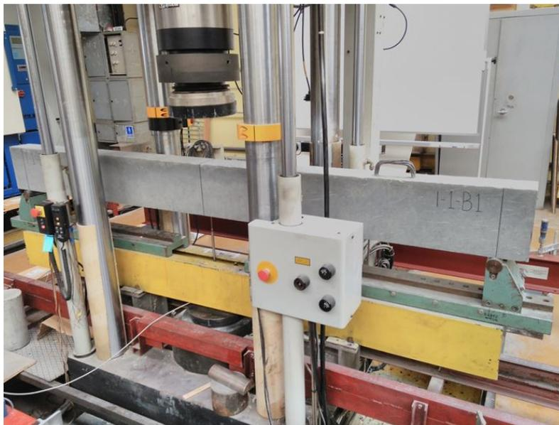
**Fig. A.1:** Full-scale beam (I-1'-B1) on test setup
