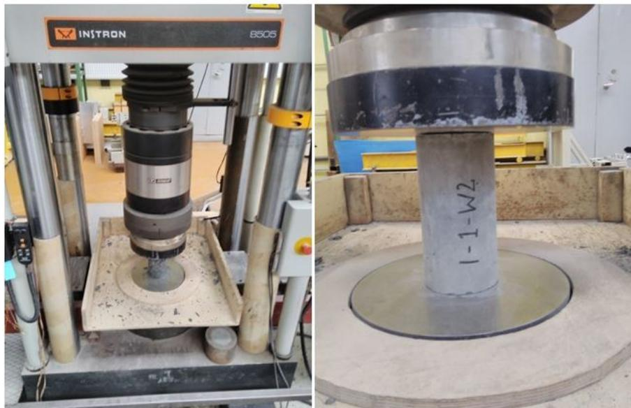
**Fig. 4.23:** Cylinder specimen mounted on compressive strength test setup
