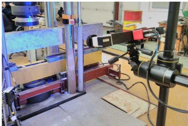
**Fig. 4.20:** Contact free measuring system ARAMIS 6M
