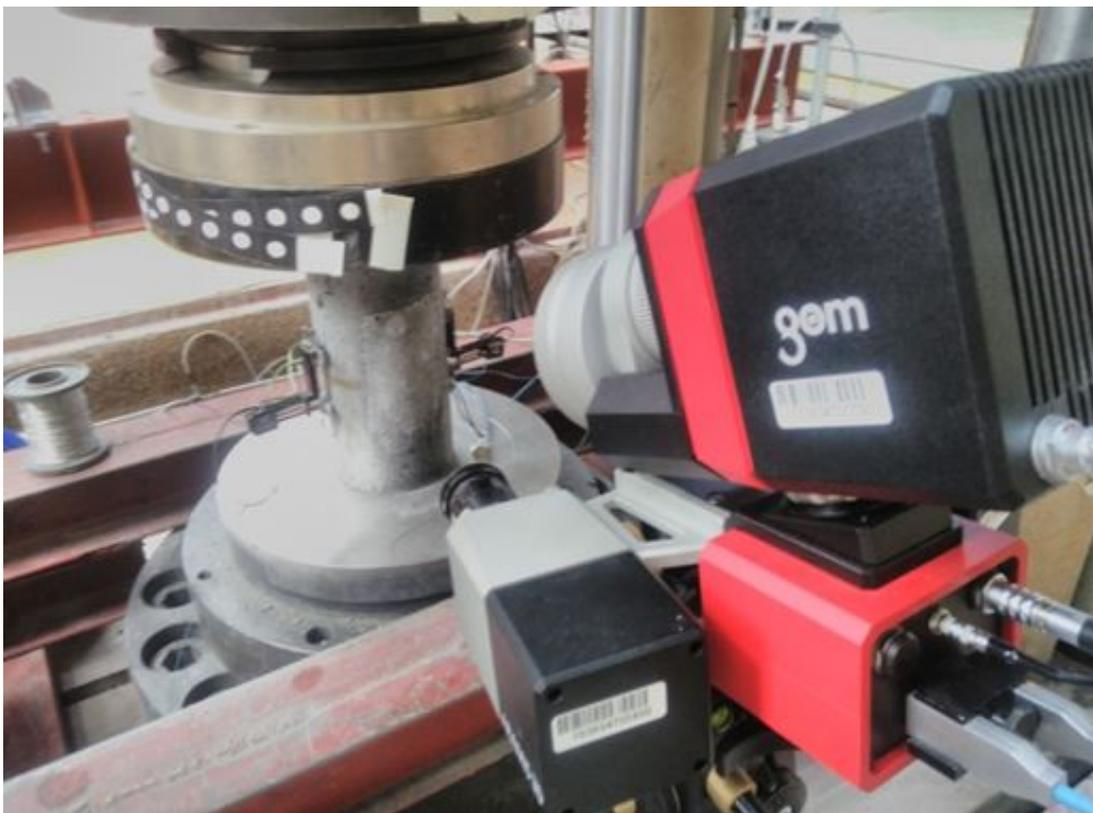
**Fig. 4.33:** ARAMIS system during the testing of modulus of elasticity
