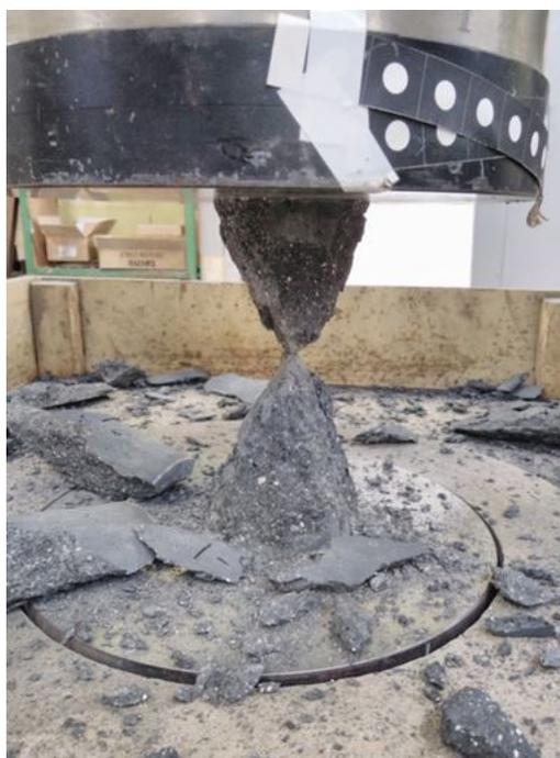
**Fig. 4.26:** The failure of cylinder under compression - specimen without polypropylene fibres (I-3-W1)
