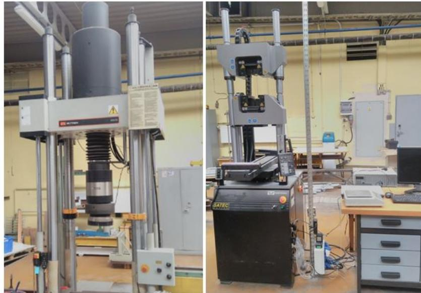
**Fig. 4.19:** Testing machines: INSTRON 8505 (on the left) and INSTRON SATEC 300DX (on the right)
