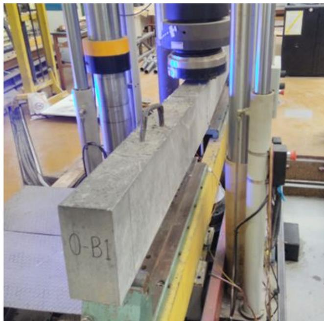
**Fig. 4.22:** Full-scale beam in a test stand subjected 3-point bending in the preliminary stage of work
