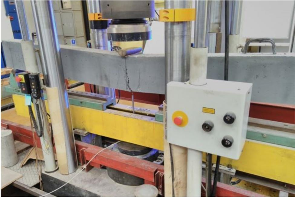
Fig. 4.41: The full-scale beam during testing
