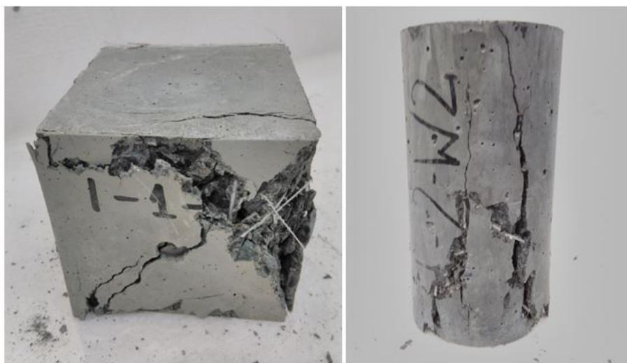
**Fig. 4.24:** Examples of specimens after compressive strength test
