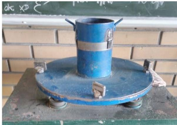
**Fig. 4.16:** Bulk density test setup
