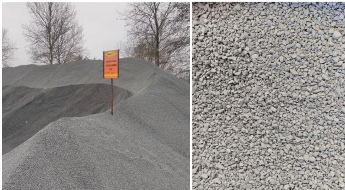
**Fig. 4.11:** Coarse aggregate (basalt) used in the research (COLAS)
