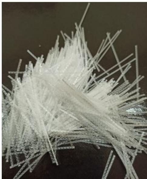
**Fig. 4.17:** Polypropylene fibre used in the research
