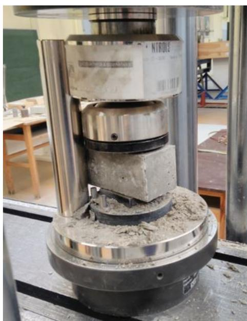
**Fig. 4.7:** Prism half during compression test
