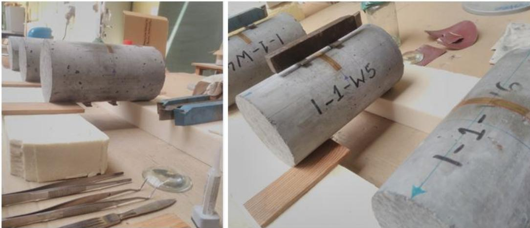
**Fig. 4.27:** Preparation of specimens for testing of material parameters
