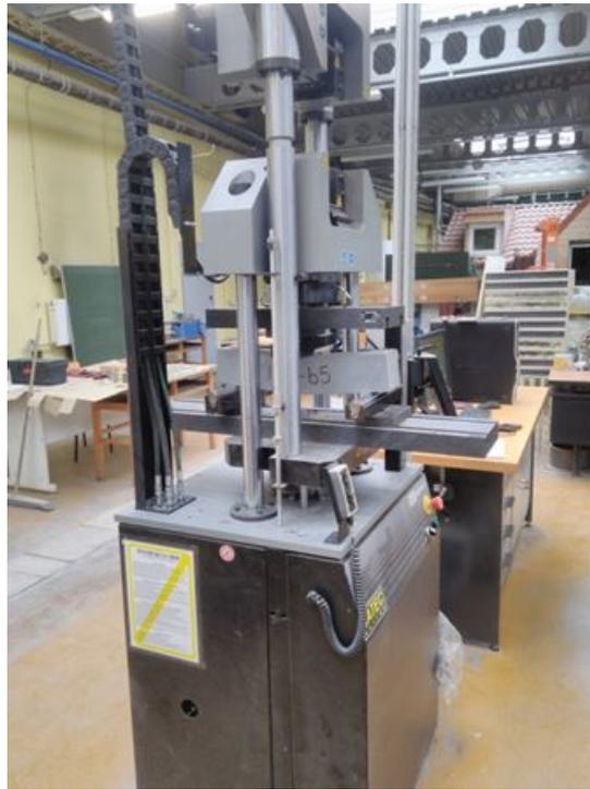
Fig. 4.35: Laboratory beam (10x10x50cm) mounted on test setup
