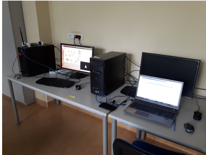
FIGURE 3.7: Photograph of the first white-space transceiver (left side computer with USRP board put on it) and REM database (right computer connected with Internet via Ethernet cable); the left-side computer communicates with database using WLAN-dongles stick into it
