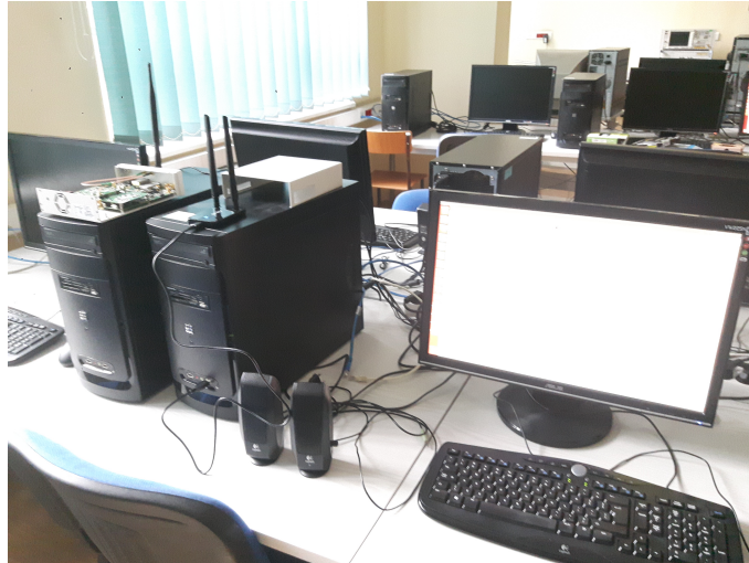
FIGURE 3.8: Photograph of the second white-space transceiver (the one with USRP board laying on it); the computer communicates with database using WLAN-dongles
