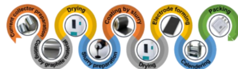
Fig. 1. Block diagram of the electrochemical capacitor production line.
