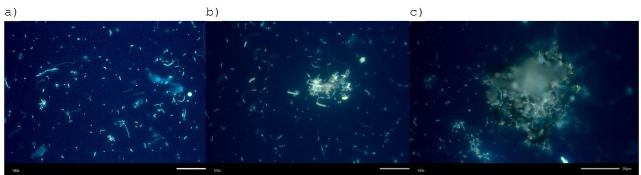
**Figure 6.** Bacteria observed under epifluorescence microscope (100x): a) morphological diversity of free-floating bacteria; b) biofilm fragments c) biofilm developed on the carbon grain
