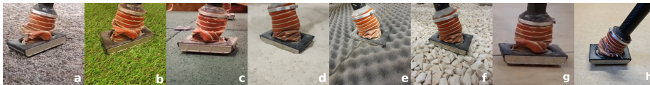
Figure 3.3: (© 2021 ELSEVIER) Terrain types included in the dataset: carpet (a), artificial grass (b), rubber (c), sand (d), foam (e), rocks (f), ceramic tiles (g), PVC (h). Each terrain gave unique F/T feedback enabling the classification of these samples.
