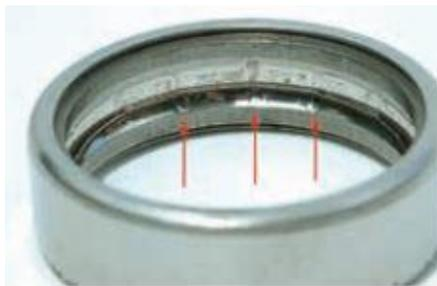
Figure 3-18: Plastic deformation at ball distance in the outer race of a ball bearing [208]
