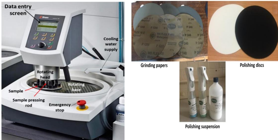
Figure 4-2: Grinding and polishing machine with its used material [247]
