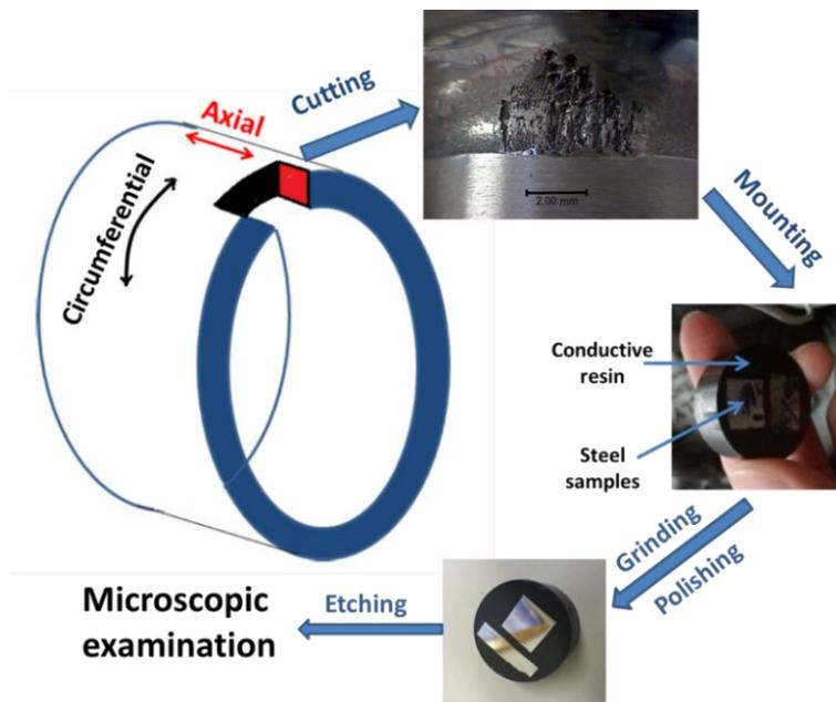
Figure 4-1: The sample preparation procedure for microscopic examination [247]
