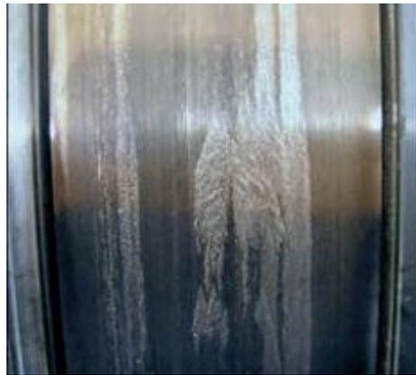
Figure 3-14: Adhesive wear at the inner raceway of a cylindrical roller bearing [208]
