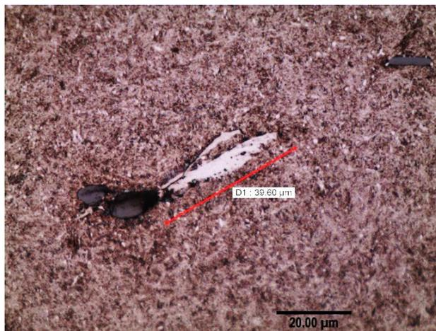
Figure 3-1: Subsurface butterfly in the inner raceway of a roller bearing [the researcher]
