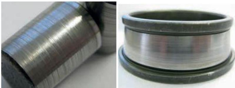
Figure 3-13: Abrasive wear on the inner raceway and roller of a Tapered Roller Bearing (TRB) [208]
