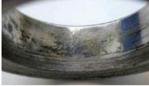
Figure 3-12: Creep of the inner ring on the shaft-seat [217]
