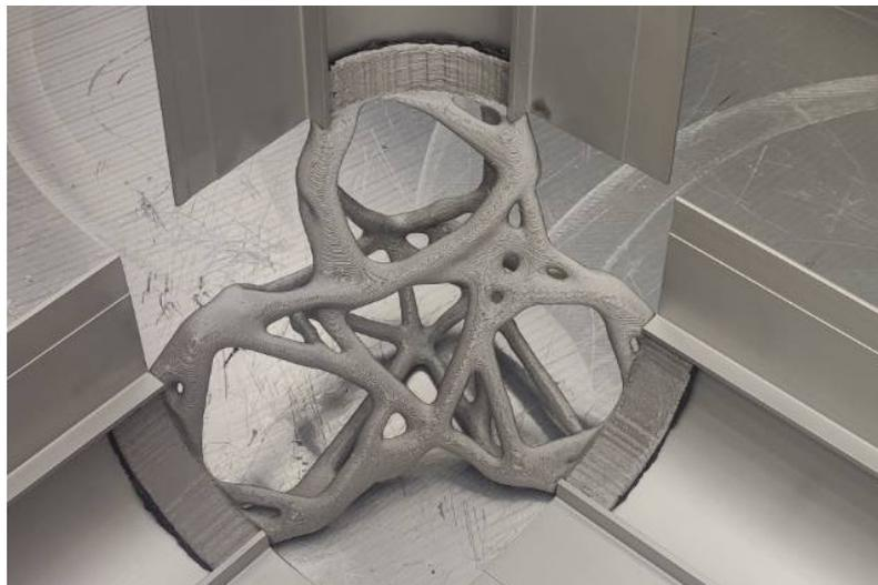
FIGURE 9.36. Photograph of one of the prototypes of the optimized box corner. This particular element has been processed with surface smoothing [18] and manufactured using FDM technology. Aluminum box edges are attached to the optimized object's edges—areas excluded from optimization.
