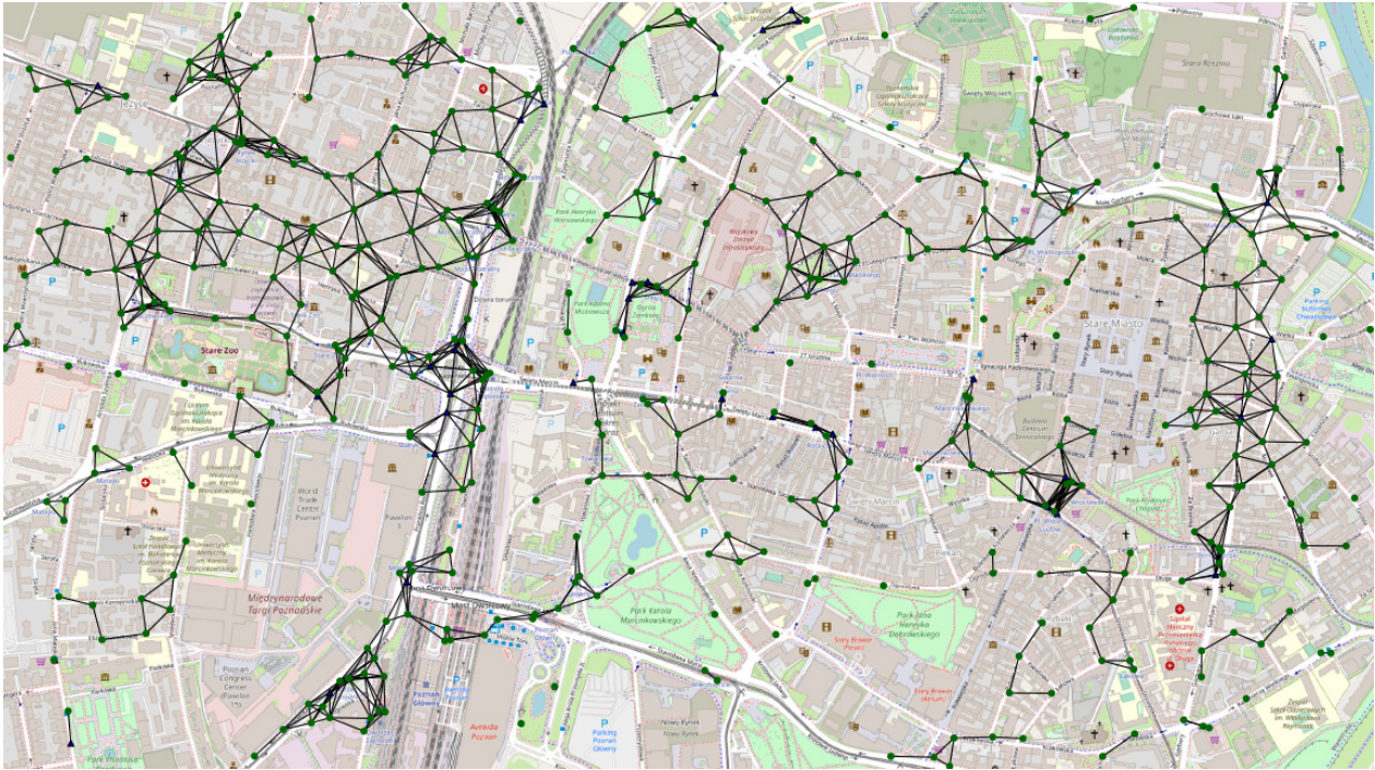
Figure 4.13 Modeled wireless connectivity graph
