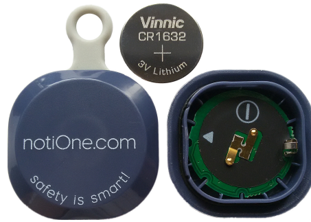
Figure 3.3 Opened notiOne beacon with a CR1632 button cell battery.
