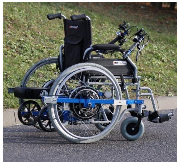
Fig 18. Prototype of a wheelchair-mounted multi-speed gear hub used in biomechanical research [P1]
