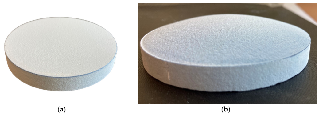
Figure 10. 8YSZ-coated 3YSZ-CNT shell-shaped composite heat-treated at 1200 °C: (a) face and (b) sides of the composite.
