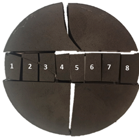
Fig. 4. Eight samples cut from a 3YSZ-10MWCNT composite shell.
